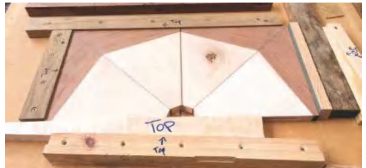
▲ Pic.16 To achieve absolute symmetry, I imitated the gap between the two door panels by laminating a strip of cherry veneer in between every eighth. Once dried and trimmed, the veneer looked very neat
